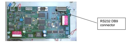
To connect the cable you have to open the cabinet and then to plug to the female connector onto the MPU card. Pay attention to push softly when you plug the connector.
