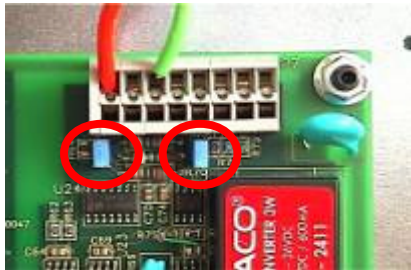
The Jumpers are set – The bus is terminated
